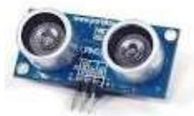
*Gambar 21 Sensor ultrasonik*
