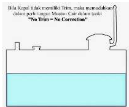
Gambar 2.8 Oil Tanker (no trim correction)
