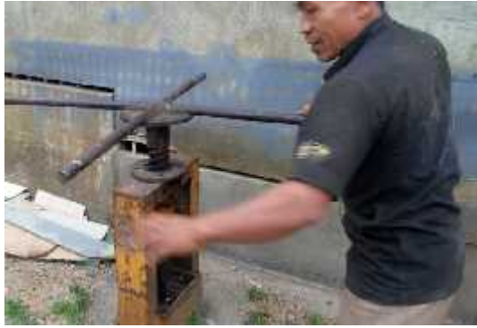
Gambar 19 Persiapan proses pengepressan/pelepasan ball joint
